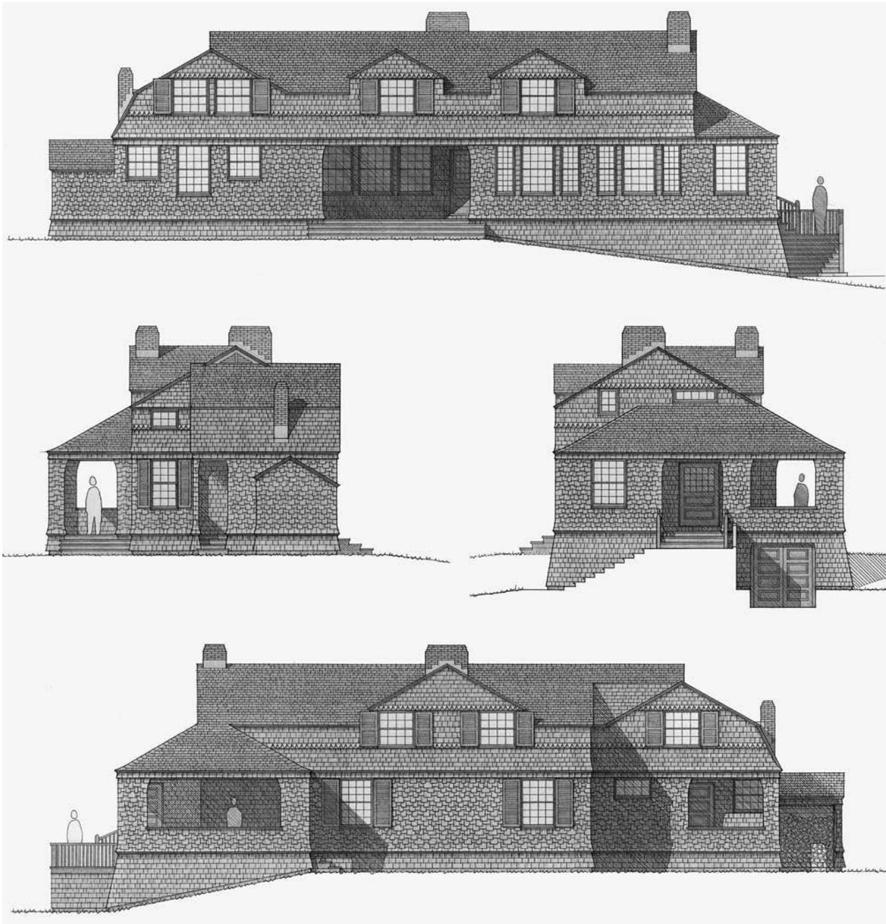
**Figure 14** Richardson, Browne house, reconstruction of elevations as built, 1882
