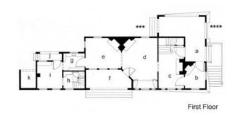
**Figure 16** Richardson, Browne house, plans as built: a. Porch and front door; b. Study; c. Hall; d. Parlor; e. Dining; f. Loggia; g. Pantry; h. Back Stair; i. Kitchen; j. Porch; k. Woodshed; l. Bath (no plumbing); m. Bedroom; n. Servant's room; + Two roof slopes steeper than 7-to-12; \* Known window with conjectural shape; \*\*Conjectural end elevation of woodshed; \*\*\* conjectural steps; \*\*\*\*Conjectural storage under porch
